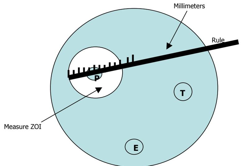
**Figure 5-4:** Measuring the Zone of Inhibition
